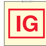
189. Inert gas installation
