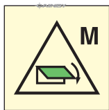
138. Remote control for closing device for ventilation inlet or outlet for machinery spaces
