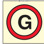
152. Emergency source of electrical power (generator)
