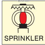
9. Space protected by sprinkler
