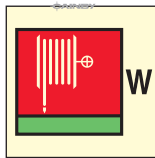
162. Fire hose and nozzle, (water)
