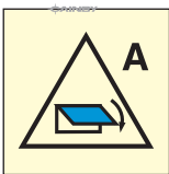
137. Remote control for closing device for ventilation inlet or outlet for accommodation & service spaces
