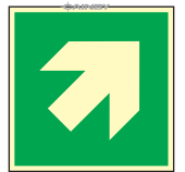
24. Means of escape diagonal directional arrow
