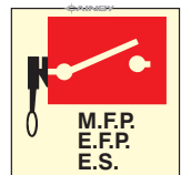
36. Remote controlled fire pumps or emergency switches
