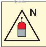
209. Remote release station for nitrogen
