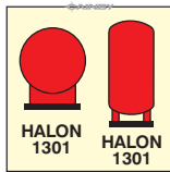
20. Halon 1301 bottles placed in protected area
